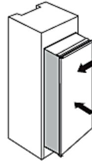
2. Screw a guide to the holes in the side of the door of the appliance using the short screws. Insert the slider into the guide, then fully open and close both the door of the appliance and cabinet to check that the door of the cabinet can close completely and smoothly.
