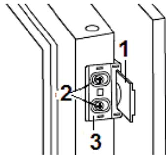
3. Open both the door of the appliance and cabinet simultaneously and mark the position of the slider when it functions well at all angle positions while closing and opening the door. Remove the slider from the guide and fix the slider on the door of the cabinet using two short screws. Then fix the slider cover.
