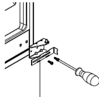
3. Move the bottom hinge pin from the right to the left side.
