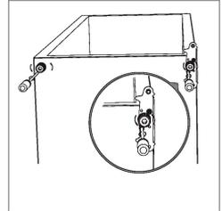
6. Unscrew and remove the bottom hinge pin,
