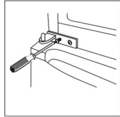
9 Place the upper door back on. Ensure the door is aligned horizontally and vertically so that the seal are closed on all sides before finally tightening the top hinge. Then insert the hinge and screw it to the front of the unit
