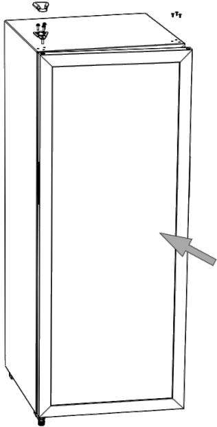
5.Align the lower hinge axle hole into the door body.
