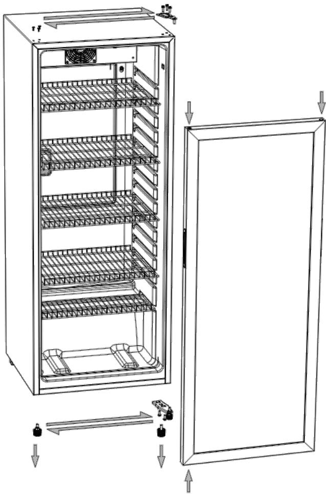
4. Remove the bottom hinge and adjustable foot.
