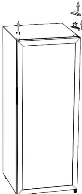
2. Remove the 3 screws for the door hinge and the 3 screw covers on the opposite side of the door hinge.
