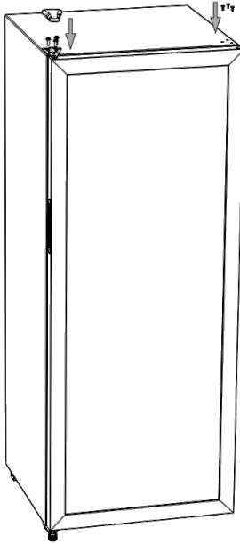
6.Screw the 3 screws on the door hinge and insert the 3 screw covers on the other side.
