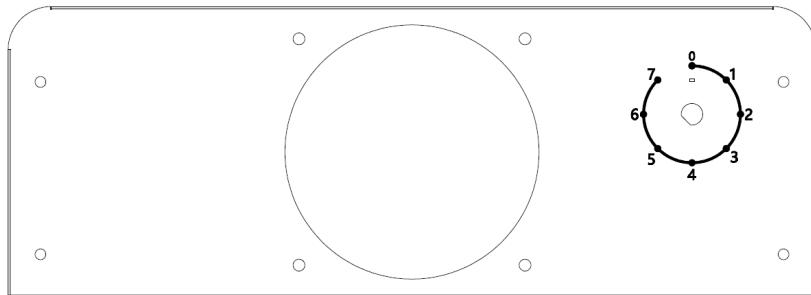
The first time you put your appliance into operation, set the thermostat to the intermediate position "3" and let it run empty for 4 hours before storing drinks so that it is sufficiently cooled. The thermostat goes from the warmest position "1" to the coldest position "7". Adjust the temperature as needed. The intermediate position "3" seems appropriate for indoor use (ambient temperature of 25°C).
