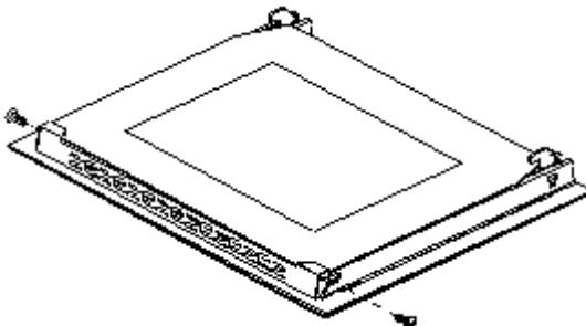
3. After cleaning, insert and block the glass panel.
