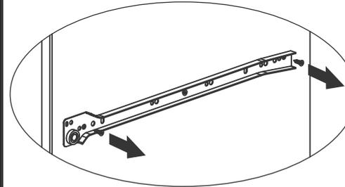
*Remove the screws on the outside of the slides that have been fixed to the side of the item of furniture. Now merely loosen the center screw.*
