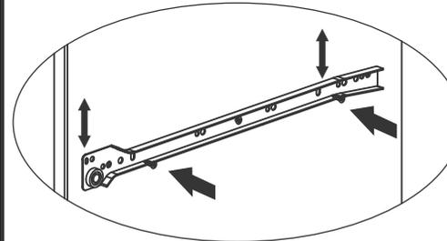
*Tighten the outermost screws at the adjustable holes of the slides. Do not tighten fully. Level out the slides as required and then fully tighten the screws.*
