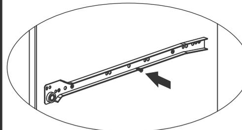
*In a last step, fully tighten the center screw.*
