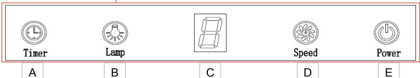
1. Press the "Power" button **E**, the button control the "on" & "off" of the hood.
