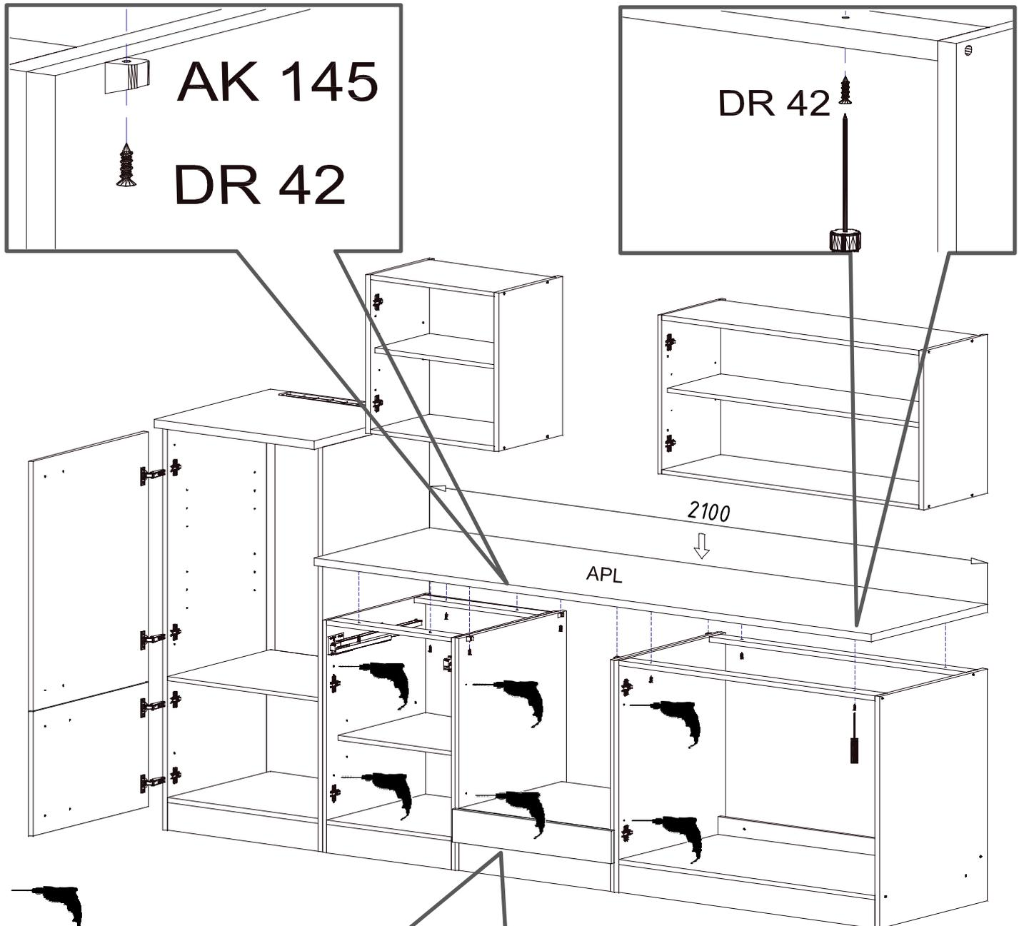
Mit  $\varnothing 5\text{mm}$  Bohrer durchbohren
