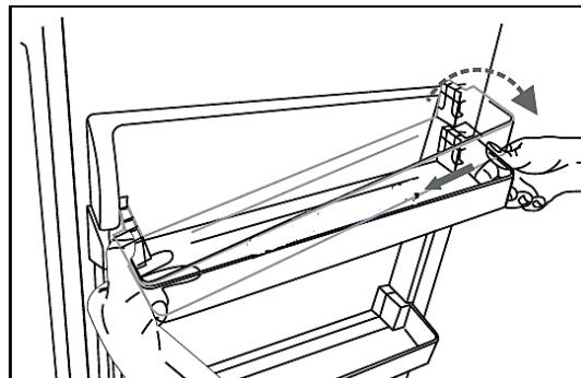
**i** The door trays can be removed and installed for cleaning as shown above.
