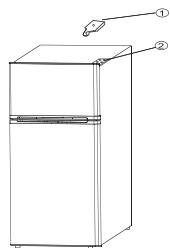
2. Lift the door upwards to disengage it from the middle hinge. Put the door to one side and lay it down gently on a padded surface.
