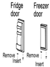
6. Place the fridge door on the lower hinge, making sure that the hinge pin is inserted in the hole at the bottom of the fridge door. Put the middle hinge back on the cabinet, making sure that it is on the opposite side from its original position.
