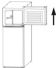
3. Using a screwdriver, dismantle the middle hinge. Lift the door upwards to disengage it from the lower hinge. Put the door to one side and lay it down gently on a padded surface.
