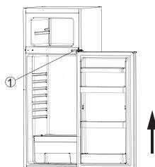
4. Swap over the position of the lower hinge and the adjustable leg to the other side of the cabinet.
