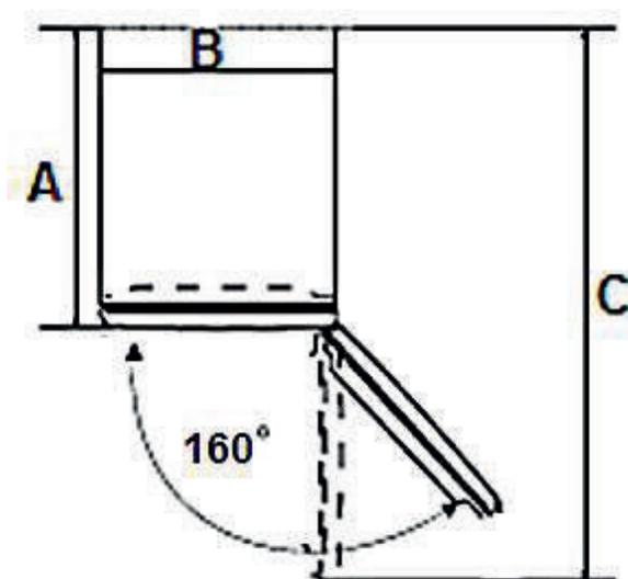
**A = DEPTH / B = WIDTH / C = DEPTH (WHEN THE DOOR IS OPEN)**
