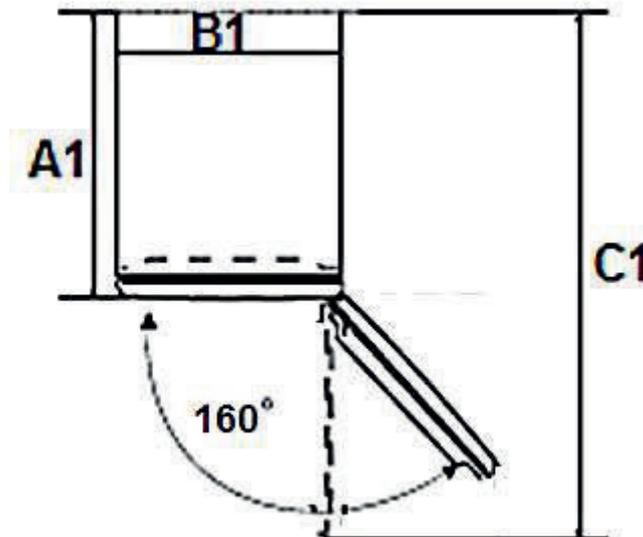
**A 1 = Depth / B 1 = Width / C 1 = Depth (when the door is open)**
