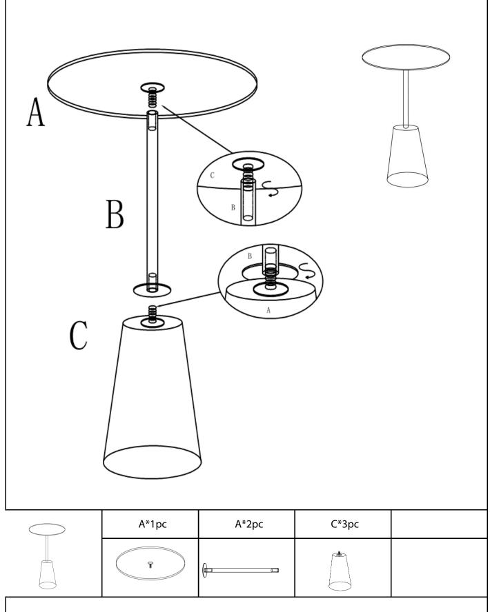
Remark: Don't Tighten any screws until item is fully assembled!
