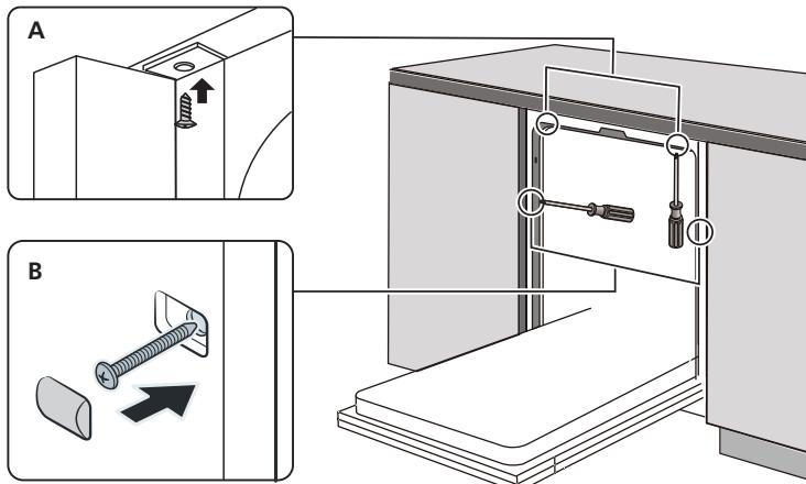
and secure it to the work surface with the screws
