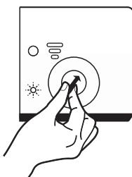
Turn the rinse aid indicator dial to a number. The higher the number, the more rinse aid the dishwasher uses. If the dishes are not drying properly or are spotted, adjust the dial to the next higher number until your dishes are spot-free. Reduce it if there are sticky whitish stains on your dishes or a bluish film on glassware or knife blades.
