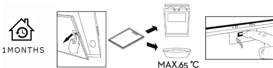
After several cleaning procedures, the colour of the filter may change. This is normal and cannot lead to replacement of the filter under guarantee. It does not affect the functionality of the hood in any way.
