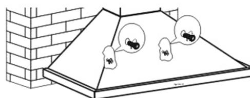
10. Fasten the air outlet cover in the exhaust air fitting of the extractor hood (if not already pre-assembled).
