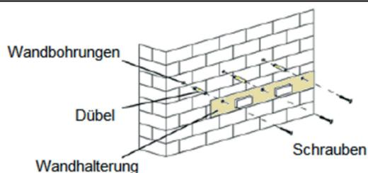
5. Hang the extractor hood on the wall bracket, hold it firmly and mark the 4 drill holes.
