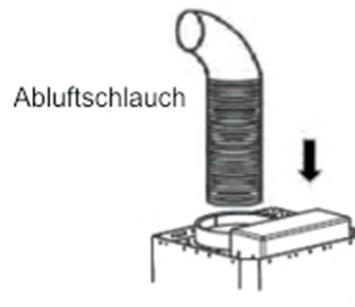
12. Insert the upper flue into the lower flue.
