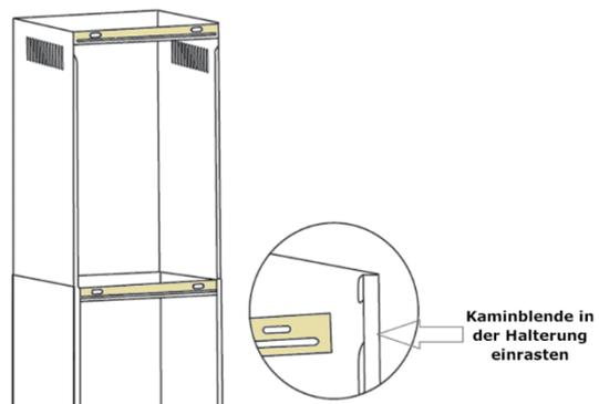
19. Connect the upper flue panel to the upper flue bracket, which is already mounted on the wall.
