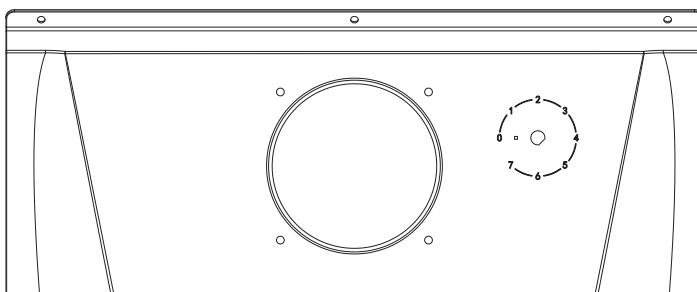
The first time you put your appliance into operation, set the thermostat to the intermediate position "3" and let it run empty for 4 hours before storing drinks so that it is sufficiently cooled. The thermostat goes from the warmest position "1" to the coldest position "7". Adjust the temperature as needed. The intermediate position "3" seems appropriate for indoor use (ambient temperature of 25°C).
